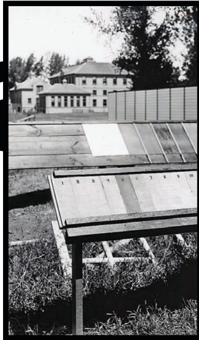
The best way to test paint in 1906? Apply it to fence posts and see how it holds up to the North Dakota elements. (Photo from NDSU Archives)
